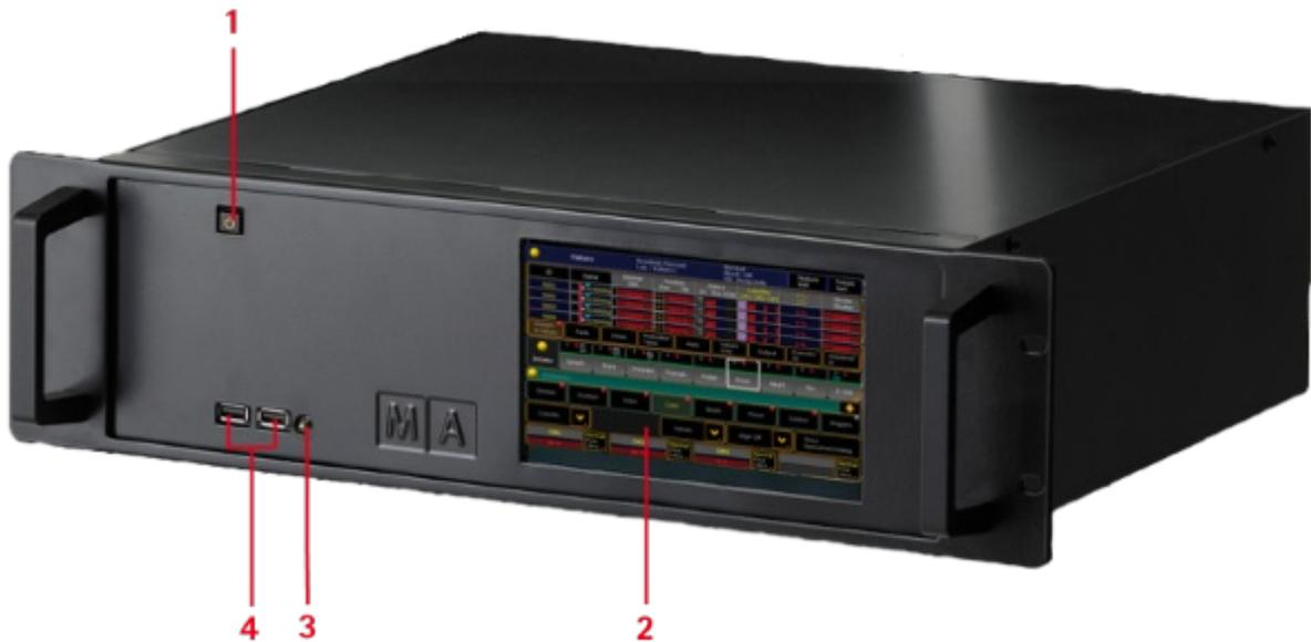
*grandMA2 replay unit (RPU) front panel*
